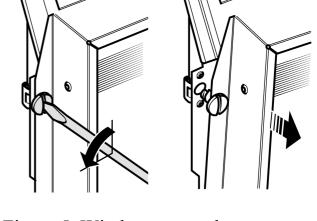
Figure 5. Window removal
